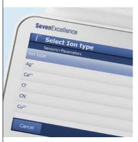
The twelve most commonly used ion types are pre-programmed in the instrument making the settings as convenient as possible. For others you can enter the ion charge and molar mass to ensure that all calculations and conversions are done for you.
