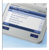
Choose from one of eight pre-defined calibration buffers groups or easily create your own. With the Pick-and-Mix™ feature you can conveniently combine pH buffers from different groups. After calibration the sensor icon shows you the quality of the calibration at a glance.
