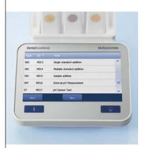
Special methods for the most common incremental ion measurement techniques are included, such as various standard addition/subtraction and sample addition/subtraction methods. This gives you a flexible and contemporary tool kit for professional ion measurements!
