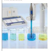
With Series it is possible to run several samples with the same method one after the other. Not only does this increase the efficiency of the analysis, but also automatically generates statistical data such as mean value and standard deviation across the samples.
